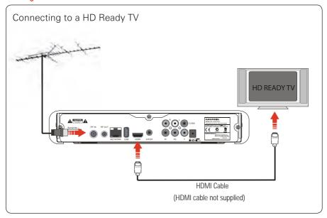
Connect the cable that comes from your aerial to the RF IN socket on the back of your Digital TV Recorder.
