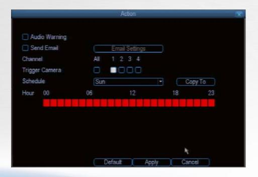
**Audio Warning:** The DVR will use its internal buzzer to emit an alarm tone. It sounds like an old computer indicating an error, or a large truck backing up.
