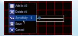
**Sensitivity:** The Sensitivity setting is controlled by a slider, allowing you to set a value between 0 and 50. The lower the number, the more sensitive the motion detection will be.
