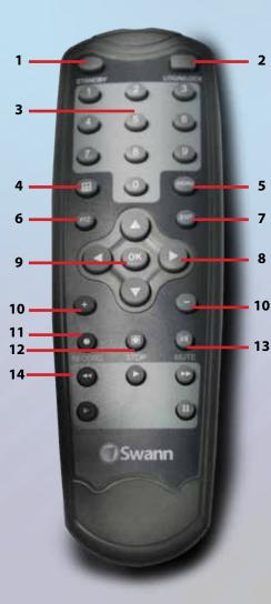
**1) Standby:** Sends the DVR into standby mode. No recording will occur while the DVR is set to *Standby*.
