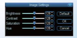
*Brightness:* Changes how light the image appears to be. However, it can't make the camera see further in the dark, or increase the clarity of an ill-lit image.
