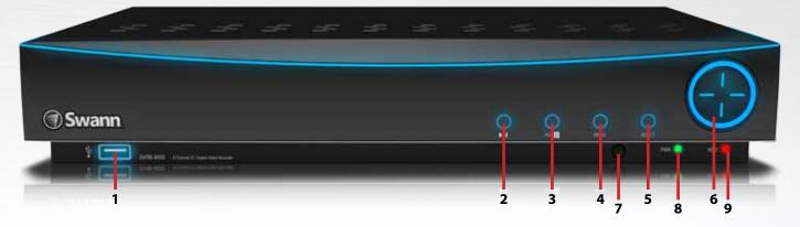
**1) USB 2.0 Port:** For connecting USB external storage to the DVR for backup, or for applying new firmware.
