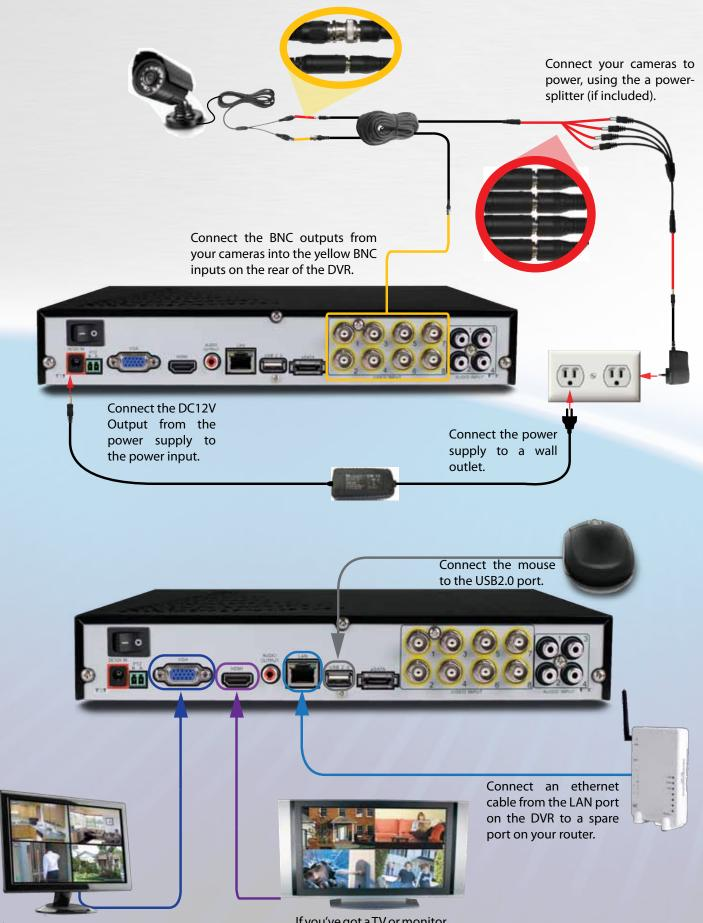
If you've got a monitor with VGA but **not** HDMI, connect it to the VGA output on the DVR.
