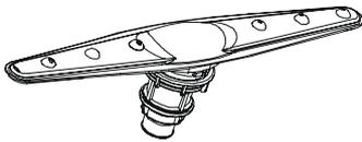
It is necessary to clean the spray arms regularly for hard water chemicals will clog the spray arm jets and bearings. To remove the spray arm, screw off the nut to take out the washer on top of the spray arm and remove the arm. Wash the arms in soapy and warm water and use a soft brush to clean the jets. Replace them after rinsing them thoroughly.
