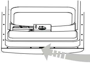
To clean the edge around the door, you should use only a soft warm, damp rag. To prevent penetration of water into the door lock and electrical components, do not use a spray cleaner of any kind.
