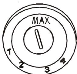
A measured amount of rinse aid is released during the final rinse. As with detergent, the amount of rinse aid needed for your dishes depends on the hardness of the water in your area. Too much rinse aid can result in lather of foaming and cause cloudiness or streaks on your dishes. If the water in your area is very soft, you may not need rinse aid. If you do, you can dilute the rinse aid with an equal amount of water.
