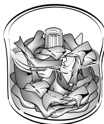
Wrong Water Level for Size of Load
