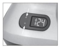
NOTE: Press and hold the arrows down to scroll through the timer setting more quickly.
