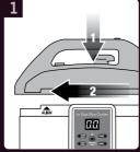
Close and lock lid in a clockwise direction by aligning arrows.
