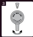
Select Pressure setting using Pressure Control Dial on lid handle (Low, Medium, High).
