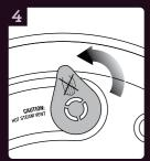
Ensure Pressure Regulator Release Valve is turned to Pressure position.
