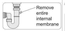
The appliance has a security feature to prevent dirty water going back into the appliance. If, the spigot of the sink has a 'non-return valve', this valve can cause the appliance to drain incorrectly. Remove the non-return valve.
