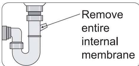
The appliance has a security feature to prevent dirty water going back into the appliance. If the spigot of the sink has a 'non-return valve', this valve can cause the appliance to drain incorrectly. Remove the non-return valve.
