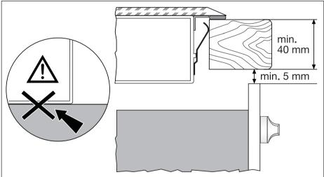
**WARNING!** Surface temperature of base exceed 95°C, under bench access must be restricted by use of non-combustible barrier on installation.
