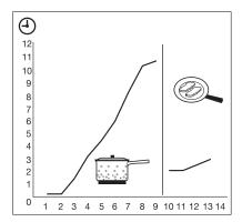
You can get a necessary heat setting in a shorter time if you activate the Automatic Heat Up function. This function sets the highest heat setting for some time (see the graphic), and then decreases to the necessary heat setting. To start the Automatic Heat Up function for a cooking zone:
