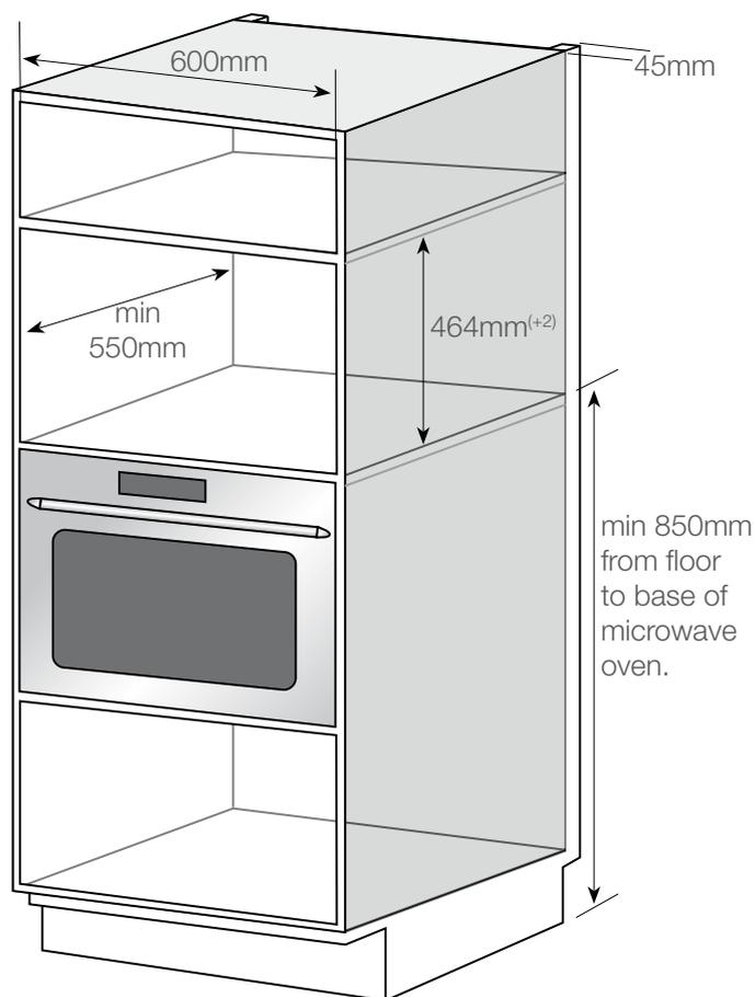
**NOTE: The microwave oven is fitted with a plug and must be only connected to a properly installed, earthed socket. In accordance with the appropriate regulations, the socket must only be installed and the connecting cable must only be replaced by a qualified electrician. If the plug is no longer accessible following installation an all-pole isolating switch must be present on the installation side with a contact gap of at least 3mm.**
