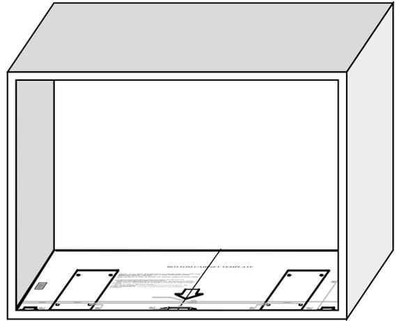
With a pencil, make marks on the bottom plane of the template according to the marks 'a' on the template.
