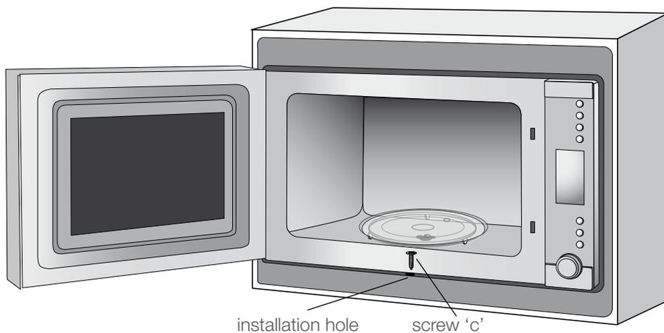
Open the door and fix the microwave oven to the cabinet with screw 'c' at the installation hole of the trim kit.
