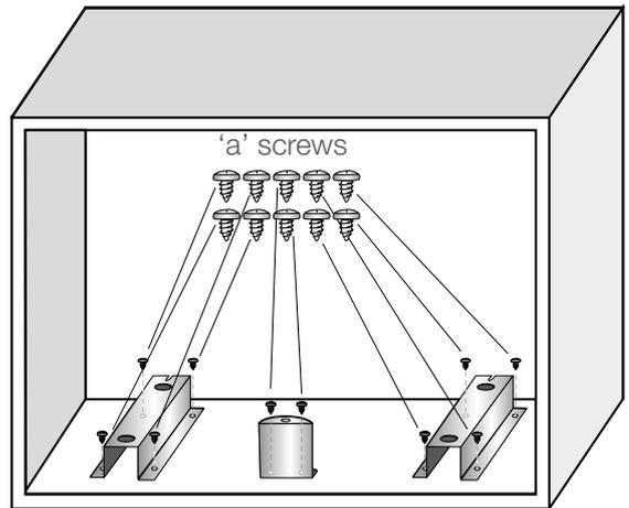
Remove the bottom cabinet template and fix the bottom brackets with screws (a).
