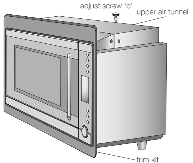
Fix screw 'b' on the upper air tunnel of the microwave oven.
