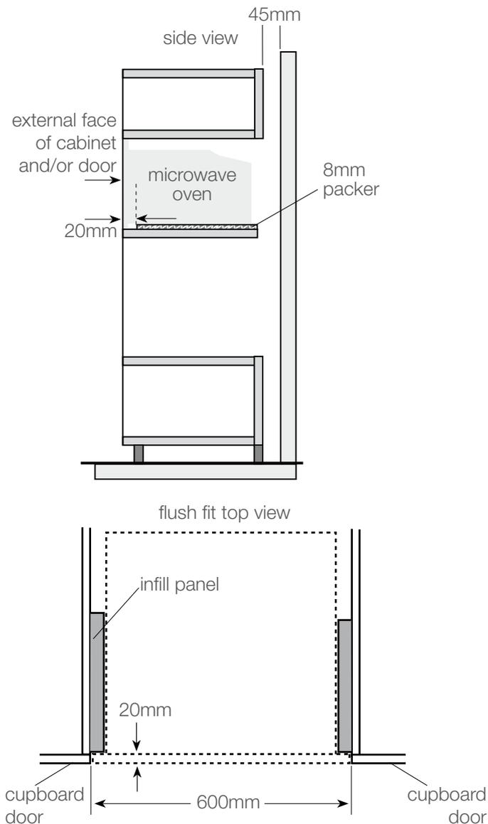
Infill panels are recessed 20mm from the external cabinet door to accommodate flush fit.
