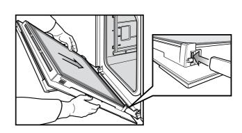
Open the door fully to access the hinges. Rotate the 'stirrups' (see the image below) until they lock into the hook. The oven door may now be closed.
