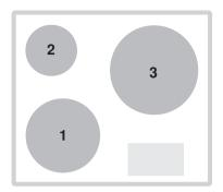
PowerPlus cannot be used with cooking zones 1 and 2 at the same time. If PowerPlus is activated with both cooking zones, then the power output is reduced for the cooking zone that was first selected.
