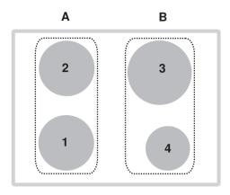
PowerPlus cannot be used with both cooking zones of a group (**A** or **B**) at the same time. If PowerPlus is activated with both cooking zones of a group, then the power output is reduced for the cooking zone that was first selected.
