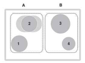
PowerPlus cannot be used with both cooking zones of any group (**A** or **B**) at the same time. If PowerPlus is activated with both cooking zones of a group, then the power output is reduced for the cooking zone that was selected first.
