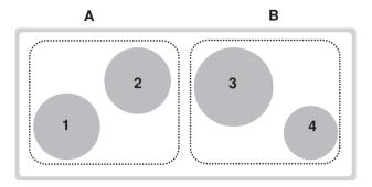
PowerPlus cannot be used with both cooking zones of any group (**A** or **B**) at the same time. If PowerPlus is activated with both cooking zones of any group, then the power output is reduced for the cooking zone that was selected first.
