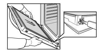
• Open the door fully to access the hinges. Rotate the 'stirrups' (see image below) until they lock into the hook. The oven door may now be closed."
