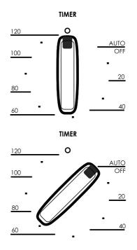
Once automatic baking is complete, return to manual operation by setting the timer to the 'OFF' mark.
