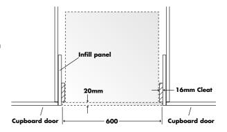
Figure A - Flush fit (top view)
