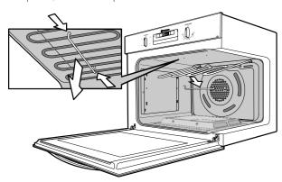
Grill in oven model shown. The grill element in separate grill models has the same hanger clip arrangement in the grill compartment.
