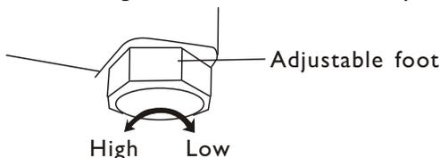
**WARNING:** Leveling of washer is very important to prevent vibration during spin.
