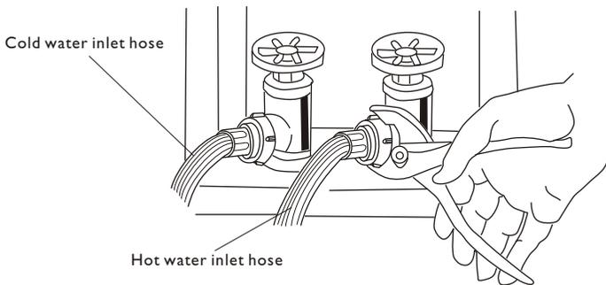
2. Connect the hot and cold water inlet hoses to the hot and cold water faucet.
