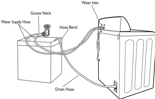
4. Plug the washer into a regular 220-240 Volt/50Hz, 10Amp outlet.
