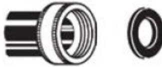
**NOTE:** You may have to use pliers to tighten the coupling. Do not over tighten because you may cause damage to the valve.
