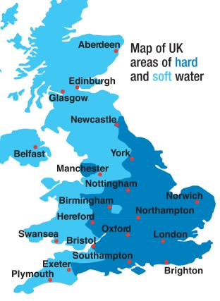
Soft water contains little or no calcium or magnesium salts, or water from which scale forming impurities have been removed or reduced.
