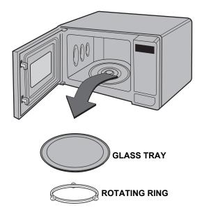
Place your oven on a flat, level surface but make sure there is at least **10 cm** of space on the top, rear and sides so there is air flow for ventilation. Exhaust outlets are located in the back and side of your oven. Blocking the outlets can damage your oven. THIS OVEN IS DESIGNED FOR AN INDIVIDUAUL BUILT IN APPLICATION. IT SHOULD NOT BE PART OF A WALL OVEN ENCLOSURE WITHOUT SEPERATION.
