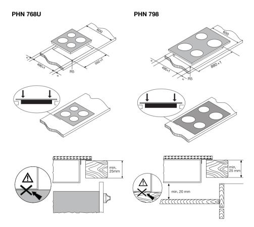
Warning! Surface temperatures of base exceed 95°C, under bench access must be restricted by use of non-combustible barrier on installation
