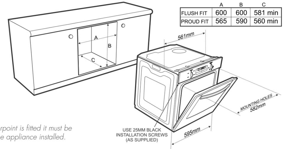
*NOTE: If a powerpoint is fitted it must be accessible with the appliance installed.*
