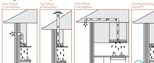
$^{\star}$  In recirculating mode you must use carbon filters to elminate cooking smells. (Model No. ARCFD)  $\uparrow$  RRE635 models are supplied with carbon filters and 70mm fascia.
