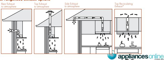
\*In recirculating mode you must use a recirculating kit which includes carbon filters to eliminate cooking smells (model no. ARCFD).
