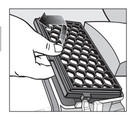
■ Fit the new exhaust filter into position.
