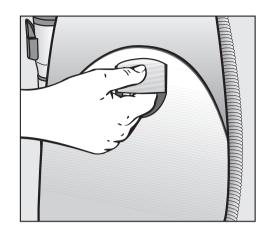
Pull on the tab at the side of the collar and swing the bag up away from the suction socket before taking it out of its holder.
