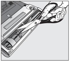
The suction hose can be opened up to clean out any heavy soiling or blockages. Any large particles inside it can then be easily removed.
