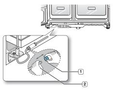
Do not cut the water line. Gently separate it from the coupler.
