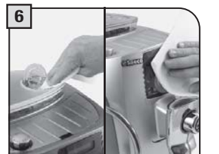
6 Clean the pre-ground coffee bypass doser with a dry cloth. Wipe the display.
