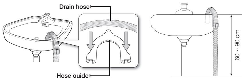
2. **In a sink drain pipe branch:** The drain pipe branch must be above the sink siphon so that the end of the hose is at least 60 cm above the ground.
