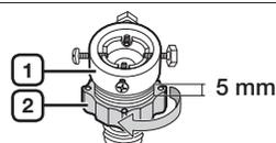
3. Connect the adaptor to the water tap by tightening the screws firmly. Turn part (2) following the arrow and connect (1) and (2).
