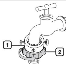
4. Connect the water supply hose to the adaptor. When you release part (3), the hose automatically connects to the adaptor making a 'click' sound.
