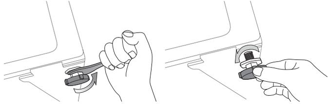
3. When your washing machine is level, tighten the nuts using the wrench supplied with your washing machine.
