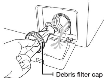
4. Wash any dirt or other material from the debris filter. Make sure the drain pump propeller behind the debris filter is not blocked.
