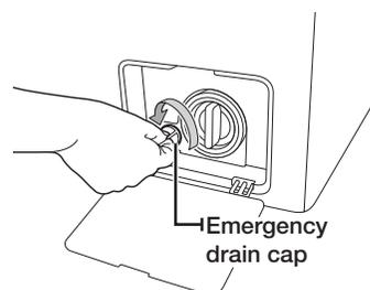
4. Hold the cap on the end of the emergency drain tube and slowly pull it out about 15 cm.
