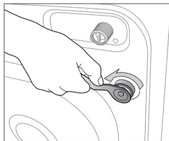
2. Hold the bolt with the spanner and pull it through the wide section of the hole. Repeat for each bolt.
