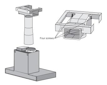
**step 4:** Carefully lower the assembled inner and outer exhaust covers onto the top of the cooker hood body, and insert the exhaust cover into the rangehood body approximately 5mm. Fix inner (top) exhaust cover to the ceiling mounting bracket with screws supplied. Ensure that the inner (top) section is extended.
