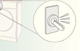
The automatic cleaning process causes a clicking noise.
