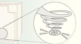
The process of pumping the condensation into the condensation container generates pumping noises.
