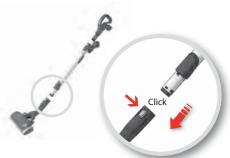
**Attach the telescopic tube to the floor nozzle** (to remove it, press the release button and pull the nozzle off).
