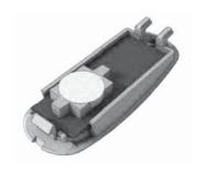
Use only batteries type LITHIUM CR2032. Batteries must be removed from the appliance before it is scrapped and are to be disposed of safely.
