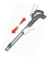
**Adjust the telescopic tube** by holding the lock and pull the handle with the other hand.
