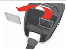
Pull the grip and remove the filter frame. Remove / Clean the filter Re-assemble filter holder by placing back in the lower part and put the frame in place at the top.
