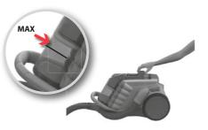
1. Dust compacting: When max level is reached, compact dust gently.
