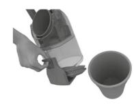
2. Unlock button and push downwards to release bottom lid.
