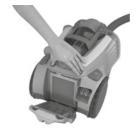
1. Press the release buttons to open the back lid.
