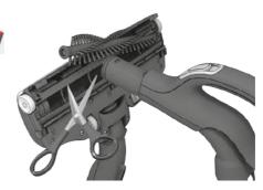
Pull out the brush roll and remove entangled threads by snipping them away with scissors. Use the hose handle to clean the nozzle. Refit in reverse order.
