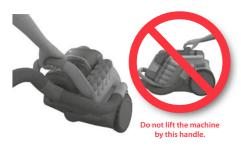
To carry machine, lift it by the handle. Do not lift the machine by the compactor handle.
