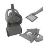
2. Remove the Pre-motor filter from the fine dust container.
