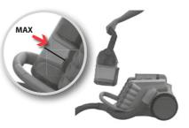
1. Dust emptying: When compacted dust reaches maximum level, lift dust container from machine by pulling the compactor handle.
