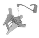
Open the fine dust container lid and wash the dust container with water. Wash the fine dust container every 2 years.
