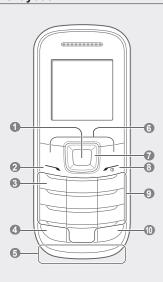
Confirm key Select the highlighted menu option or confirm an input; In Idle mode, access Menu mode
