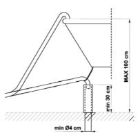
The free end should be positioned at a height of between **30 and 100 cm**, and should never be submerged in water. If a horizontal drain extension hose is used (for a maximum of 3 m) the drain hose can be placed at a maximum height of **85 cm** from the ground.
