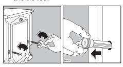
2. Remove the bottom cover placed into the drum of your appliance, lay it's hook as the arrow 'A' indicates and push the top of the cover to seal it closed.
